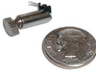
The operation of a DC motor is based on the magnetic field generated when an electrical current flows in an inductor. Hence, by controlling the current flowing through the motor, we can adjust the motor speed. This can be done by varying the driving voltage or switching on and off the current to the motor using a pulse width modulator.
