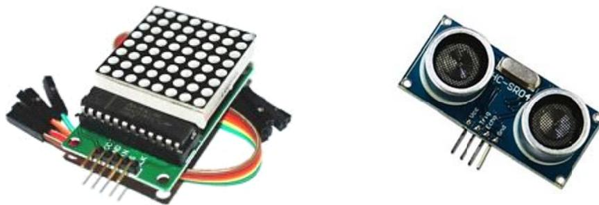
Your program needs to create an animation by displaying a sequence of patterns on the LED matrix. To display a patten, 8 bytes of pattern should be written to the driver chip via SPI interface bus. Assume we will use the example definition of a patten:
