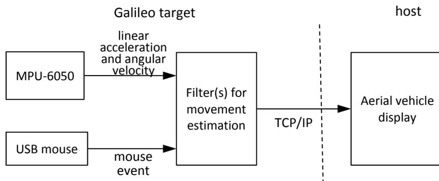
When your program begins to run, the MPU-6050 accelerometer and gyroscope sensor module should be configured properly and initialized with a sampling rate of 200, approximately. Then, your program can read in a stream of accelerometer and gyroscope rate data and estimate the position and orientation of the rigid body. To estimate position changes, you can perform double integration of acceleration data in X, Y, and Z axes. For orientation, you can
